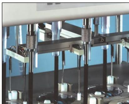
AutoTemp and Automatic Dosage Delivery Module
