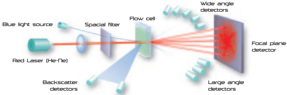
The Mastersizer 2000's wide dynamic range and flexible operation are achieved through Malvern's capacity to precisely engineer and optimize the system according to the physics of light scattering.
